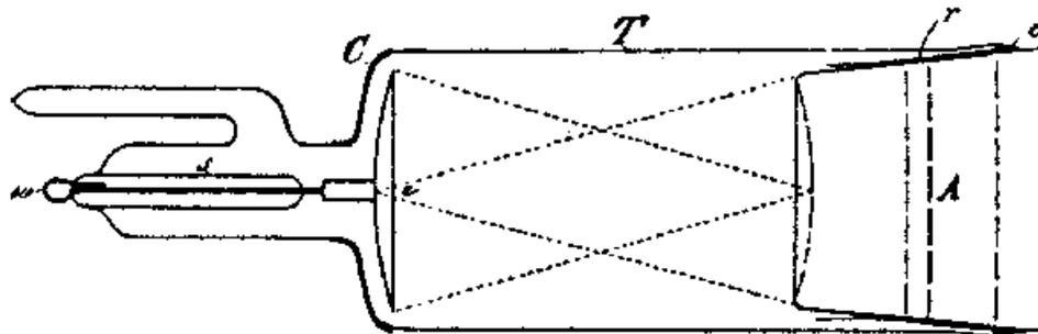
Figure 5: One of Tesla's Roentgen tubes with one single electrode (from [32]).
