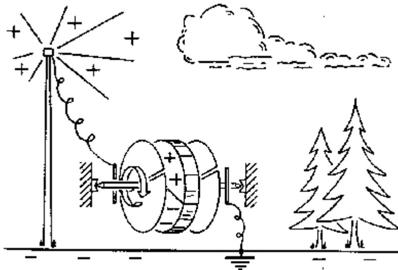
Figure 9: Driving an electrostatic motor with the positive electric field of the atmosphere; from JEFIMENKO Oleg D., *American Journal of Physics* **39** (July 1971) p.777
